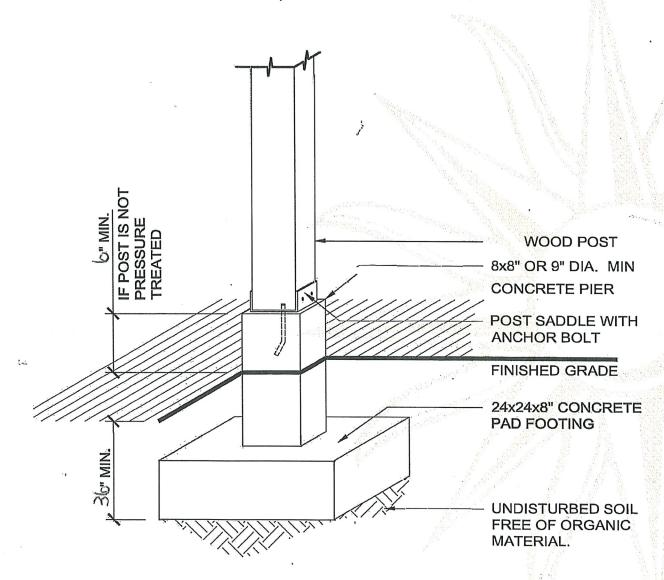
FOR UNFACTORED LOADS LESS THAN 8350 LBS. WITH 2088 PSF MIN. BEARING CAPACITY
